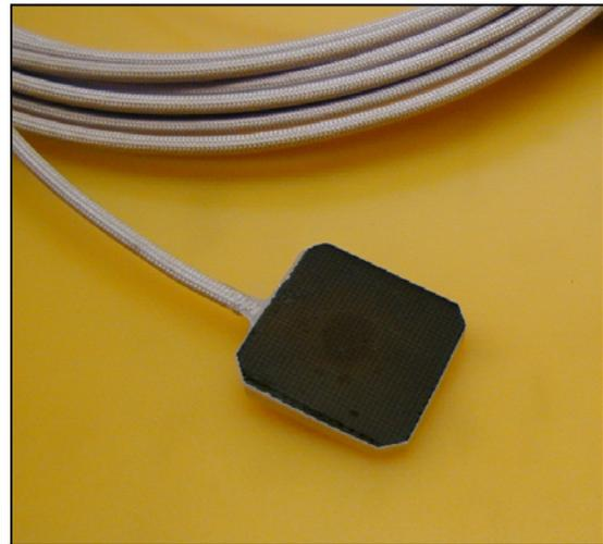
Example of a Thinline Flux Probe for use in Salient Pole Rotors.
